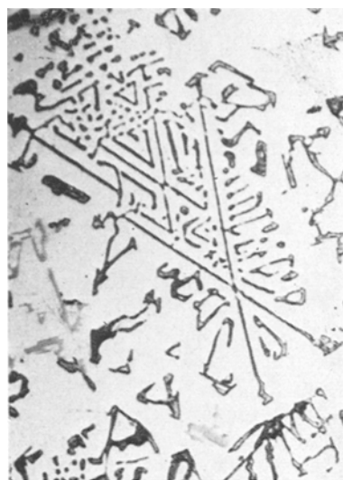
Figure 4 \alpha Al-Mg_2Si eutectic in longitudinal section ( \times 450 ).
