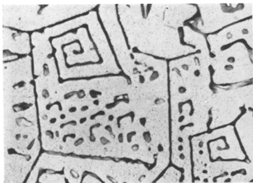
Figure 2 Spiral eutectic of \alpha Al-Mg_2Si in Al—Mg—Si alloy ( \times 550 ).
